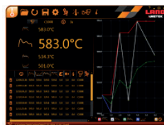
The Table View showing Instantaneous, Valley, Average and Peak, plus the unique Meltmaster temperature (on the 055 L model) readings.
